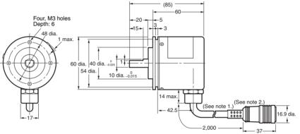
Note 1. 6-dia. 12-conductor oil-resistant PVC insulated shielded cable, (conductor cross-sectional area: 0.2 mm<sup>2</sup>; insulator diameter: 1.1 mm dia.), standard length of 2 m
