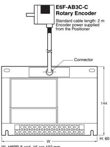
W: H8PR-8 and -16 are 192 mm H8PR-24 is 240 mm Simplified Key Switch H8PR-8, -16, and -24 Rotary Positioners
