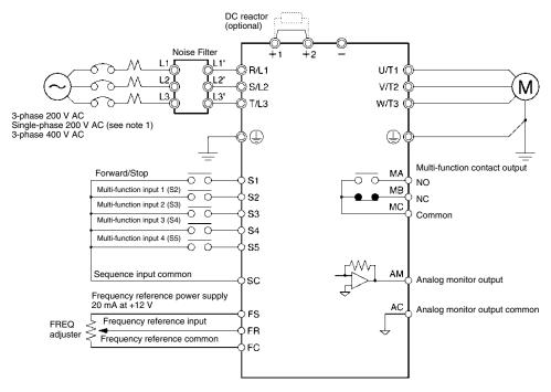
Note: 1. Connect single-phase 200 V AC to terminals R/L1 and S/L2 of the 3G3JV-AB ...
