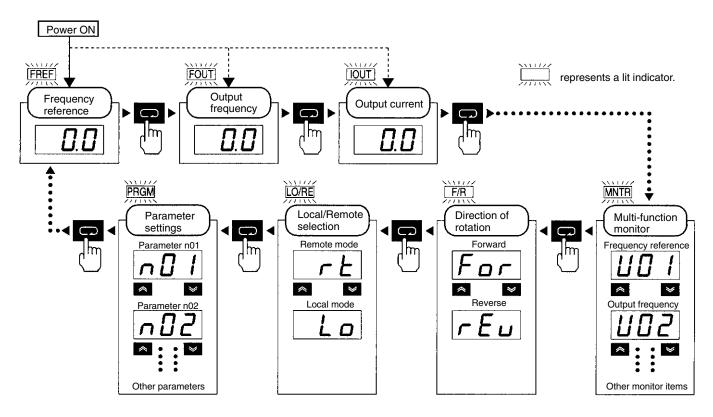
**Note:** If the power is turned OFF with the FOUT or IOUT indicator lit, the same indicator will light when the power is turned ON again. In other cases, the FREF indicator will light when the power is turned ON.
